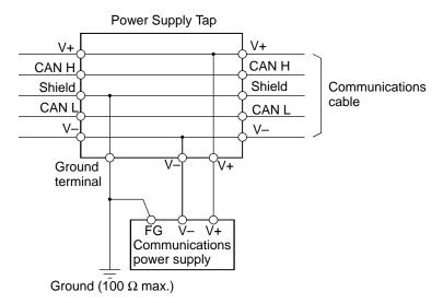
If more than one communications power supply is connected to the same Network, ground only the one nearest the center of the Network. Do not connect the shield wire at the other power supplies.
